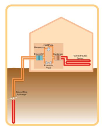
Figure 1: A typical GSHP system
