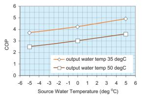
Figure 5: Coefficients of performance of typical small GSHP's
